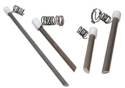
Available in **SEVEN** different sizes and styles ranging from 1/2 lb. to 3 lbs., the "Husky" Drive-in anode is the easy, reliable way to protect natural gas service lines. One man can install the "Husky" in minutes with only a hammer and screwdriver. With the "Husky", you just "drive it in" and connect the wire lead to the service line.
